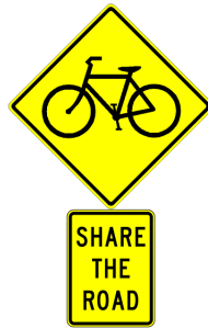
Figure 4-10: Typical Warning Signs (W11-1 and W16-1P)
